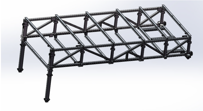
Figure 3. Schematic diagram of movable arch frame
